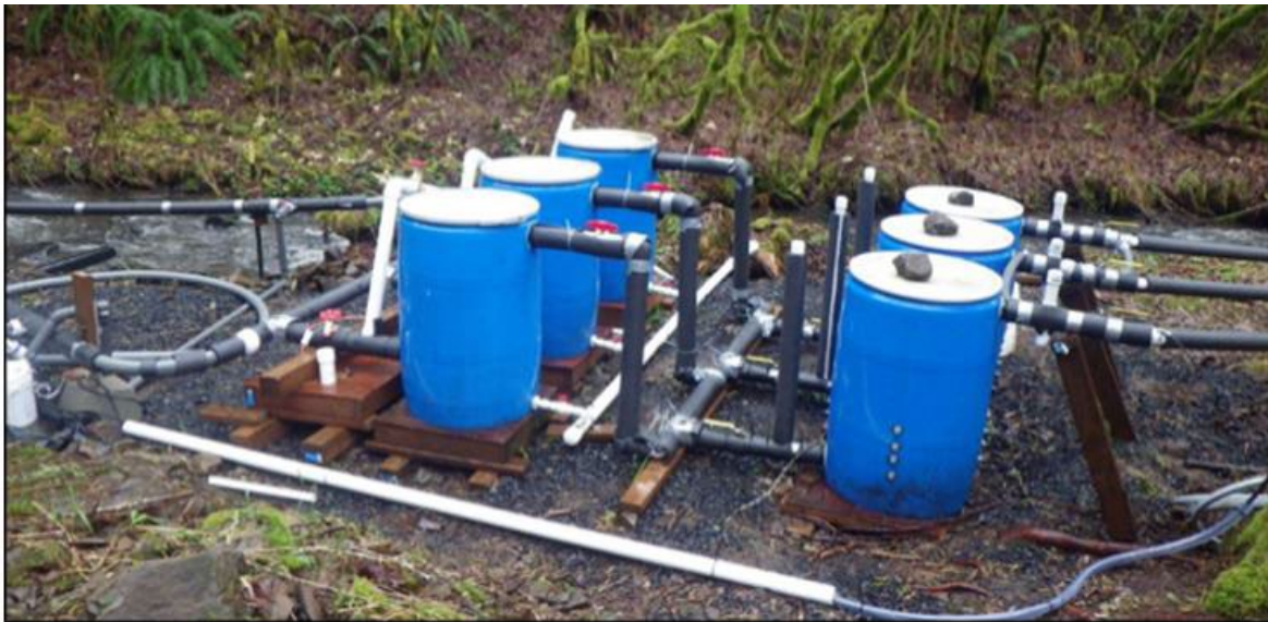
Figure A-II: 1. Remote-site Incubator (RSI) installed at Perkins Creek, Oregon, for outplanting chum salmon eyed-eggs. In this photo, water enters the sediment settling barrels on the left side and flows out of the egg barrels on the right side.
