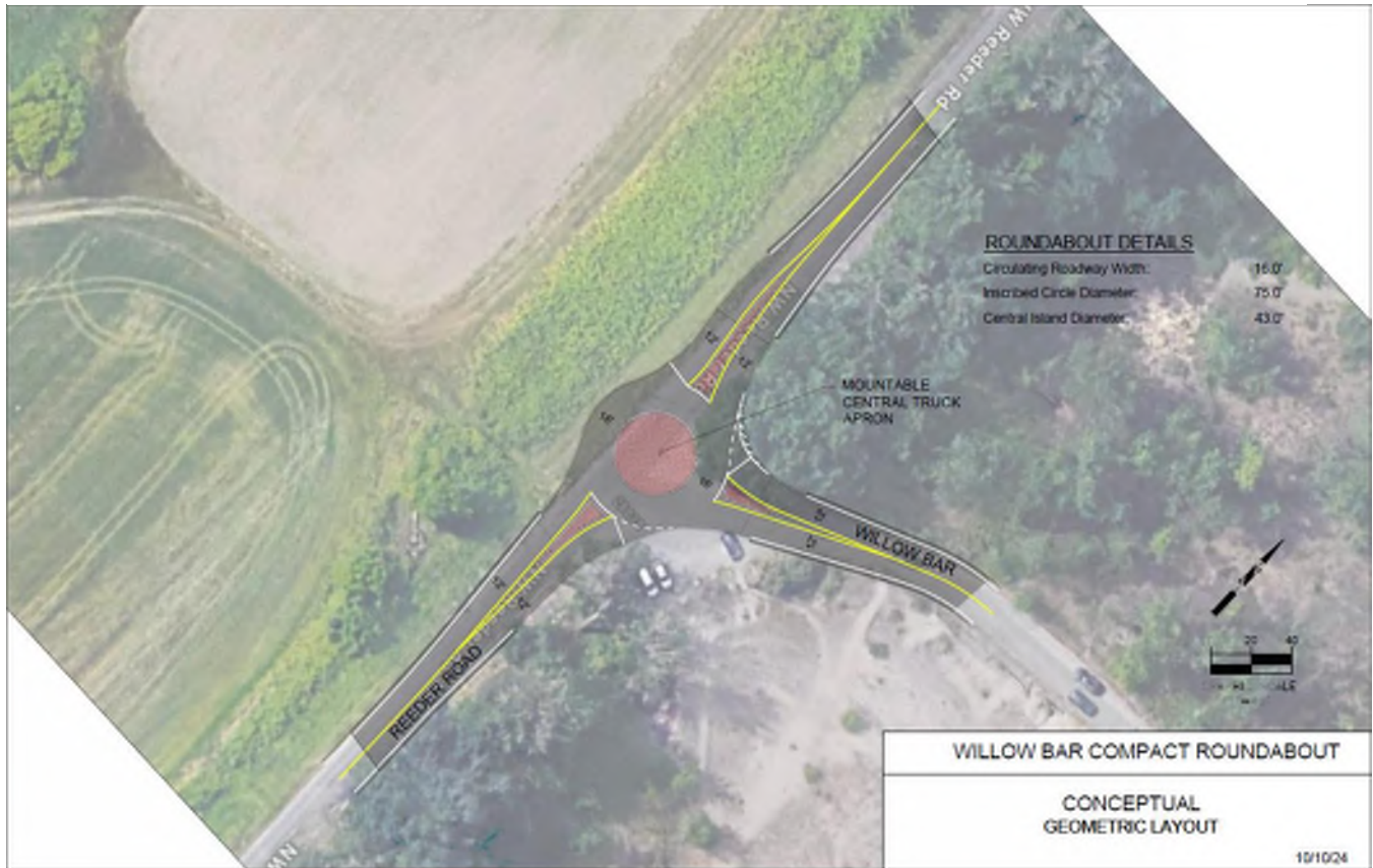
Figure 5 - Possible Willow Bar Compact Roundabout (Source: DEA)
