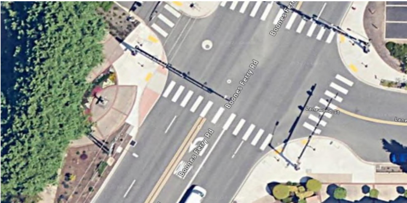
Figure 8 - Aerial View of U-Turn with Apron (Source: maps.google.com)
